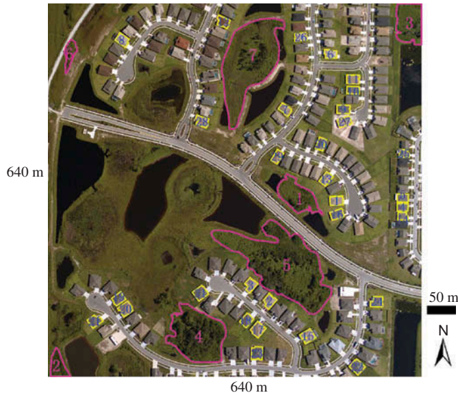
Figure 5. The aerial image used for segmentation and quality assessment. The yellow-bordered polygons are the AIRs of the buildings; the purple-bordered polygons are the AIRs of the forests; the blue numbers are the codes for buildings; and the purple numbers are the codes for forest.
